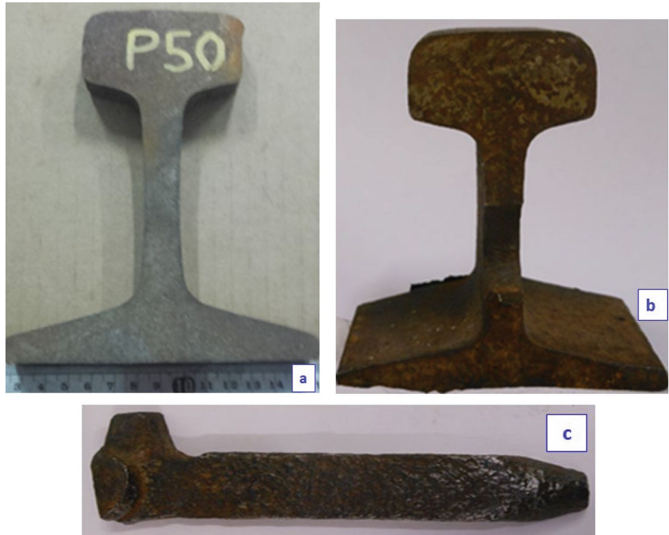
Fig. 1 (a) P50 rail wide gauge 1520 mm of Sovietic origin; (b) 750 mm narrow gauge rail of German origin; (c) fixation nail of Belgian origin
